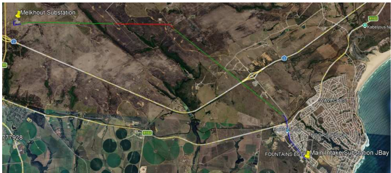
Figure 1. Route of existing 66kV overhead line. Blue – Phases 1 to 3 previously completed. Red – Approx. 2,3km this tender. Green – Future
