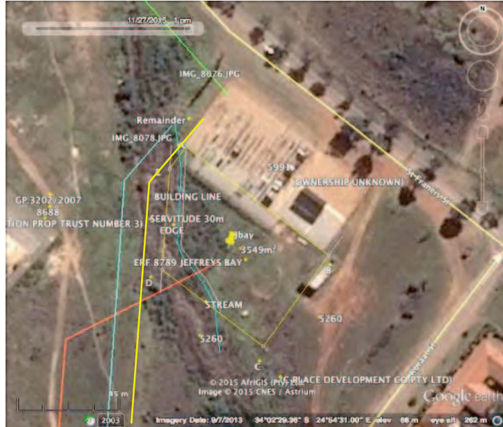
Figure 5: The blue line depicts the actual surveyed edge of the stream. The white line to its right is the building line and identified the area to its left where no construction is allowed. From the white line to its right is the expansion area.
