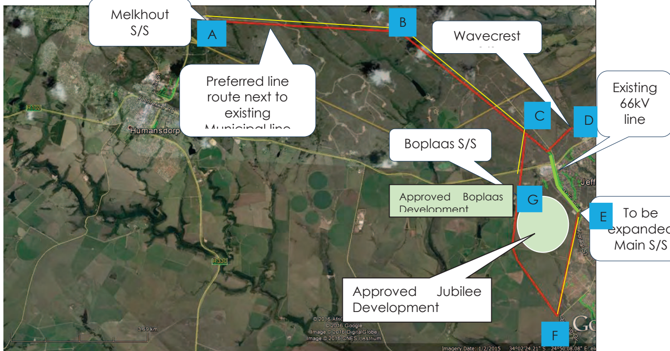
Figure 1: Locality and Layout of proposed project showing the preferred (red) and alternative (blue) route with the existing 66kV powerline in green
